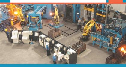
**USAI FORGE Pvt Ltd** is a fully automated and robotized closed die forging facility with the latest Induction Heating System and series of Forge equipment. Facility is located 90 kms from Hyderabad on NH 65. Covered area is 50,000 sft including the Forging Facility, Precision Machining Facility and Flow Forming Tubes Facility. Clean room assembly is specifically designed for the assembly of high precision engineering components.
